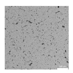
**TEM.** Transmission electron microscopy of sonicated Alpha-synuclein Protein Pre-Formed Fibrils (PFF).
